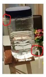
Put a plastic bottle on the support tower and glue it to the wooden base with a thermo gun. On a plastic bottle, drill one hole at the bottom of the bottle to put a straw in it. Drill the second hole on top of the bottle on the other side of the bottle and also insert a straw there. Seal it the straws with thermo gun.
