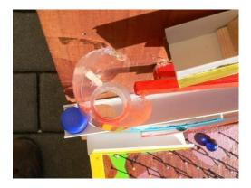
After falling down-through the hole of the groove, the marbles roll over the circular path to the lower edge, where the path along Marjanca (name of the device) continues in the middle. The bottom part can also be concluded in other different ways. Some suggestions: marbles travel between the stoppers of bottles, marbles travel between short inclined tiles, etc.
