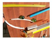
We deliberately leaned the first step to create a "pocket" for the marble. Marble which rolls on a sloap, clash into a stationary marble and stops, while the stationary marble rolls ahead (presentation of the physical law of the collision of two identical balls).
