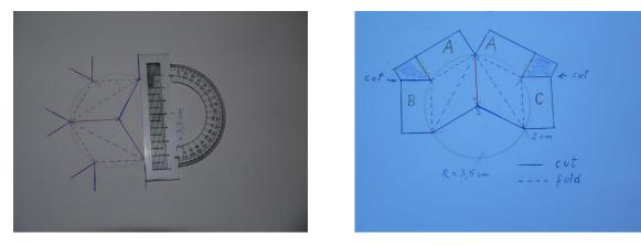
Cut out the image along the solid line. The dashed lines indicate only paper folding. Inside the image cut only along the line marked with a »cut« in the picture.
