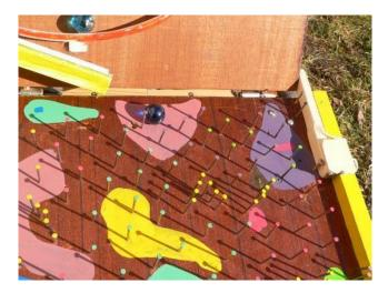
At the bottom of the Marjanca, we made rectifiers, which direct the ball into the middle. In the middle, we left an opening of 5 cm wide. Through the opening, the marbles are falling into a plastic box. Box prevents the marbles from rolling uncontrollably over the room. The tilt of the rectifiers is 15 degrees to the bottom edge of the board.
