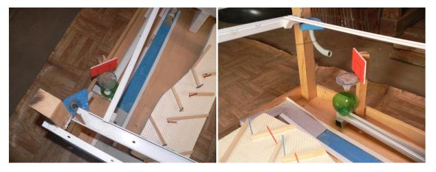
Through plastic groove (they represent the marathon run track), we lead the received ball at the entrance of the device to the opening of the curved plastic tube carrier to the basket. The ball comes into the contraption at a height of 44 cm. The plastic tube is 1.1 m long and is removed during transport, so that the dimensions of the device are smaller. The cross-section of the tube is 4 cm x 2.5 cm, but it can also be 3 cm x 2.5 cm.
