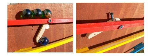
The ball starts to roll along the yellow slope to the red feeder. The feeder is made out of the cork. The purpose of the feeder is to deliver a single marble from one to the other slope and at the same time preventing the rolling of several marbles in the group. We removed the slats of slopes from the base plate so that the marbles roll over the edge of the slats in the gutter.
