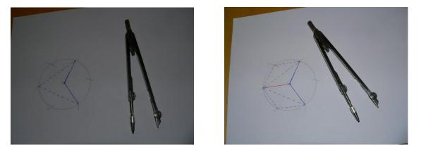
Draw the rectangles on the dashed lines connecting the adjacent points on the circle (also obtained as an extension of the side of an equilateral triangle, as shown by the geometric triangle side in the figure below). The rectangles are 2 cm long (slightly higher than the wall). Connect the ends of the rectangles with a solid line and finally draw as shown in the picture below.
