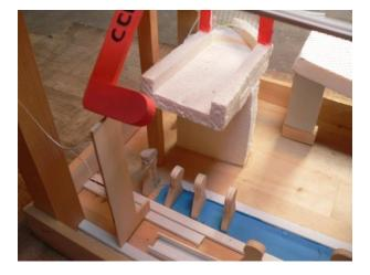
The slope (representing the rowing track) is made from a plastic groove, which is 4 cm wide, 2,5 cm deep and in our case 85 cm in lenght. At the beginning of the slope, under the basket, we can attach a cut-off funnel of a plastic bottle to ensure that the ball from the basket drops safely into the groove.
