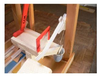
We have to move the hockey stick from a balanced position and support it with a wooden sling. In our case, the height of the slat is 22,5 cm. When the ball falls through the basket, it rises to the wooden sling on the slope and pushes it under the hockey stick, so the stick swings and hits the ball in the goal.
