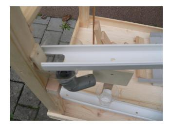
The slope (representing the rowing track) is made from a plastic groove, which is 4 cm wide, 2,5 cm deep and in our case 85 cm in length. At the beginning of the slope, under the basket, we can attach a cut-off funnel of a plastic bottle to ensure that the ball from the basket drops safely into the groove.
