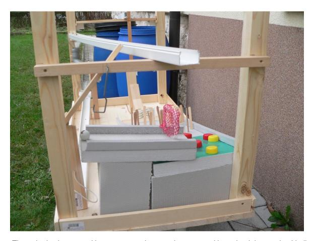
Through plastic groove (they represent the marathon run track), we lead the received ball at the entrance of the device to the opening of the curved plastic tube carrier to the basket. The ball comes into the contraption at a height of 44 cm. The plastic tube is 1.1 m long and is removed during transport, so that the dimensions of the device are smaller. The cross-section of the tube is  $4 \text{ cm } \times 2.5 \text{ cm}$ , but it can also be  $3 \text{ cm } \times 2.5 \text{ cm}$ .
