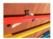
The ball starts to roll along the yellow slope to the red feeder. The feeder is made out of the cork. The purpose of the feeder is to deliver a single marble from one to the other slope and at the same time preventing the rolling of several marbles in the group. We removed the slats of slopes from the base plate so that the marbles roll over the edge of the slats in the gutter.
