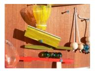
The three pendulums show the transfer of energy in collisions between solid bodies. The horizontal force of the marble in a collision with wooden balls is transferred through wooden balls to a marble that is mounted on screws. The marble ran into a white gutter.
