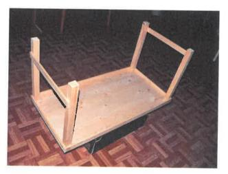
Attach the base columns to all four corners of the baseboard from below with screws (5 to 7 cm long) upright posts. One screw in the middle of the pillar is sufficient. When we position the columns, care must be taken that they are spaced from the edges as far as the thickness of the slats that will connect the columns to each other. Before screwing the columns with screws, it is advisable to grease the contact surface with glue. Place the battens that connect the columns on the base board
